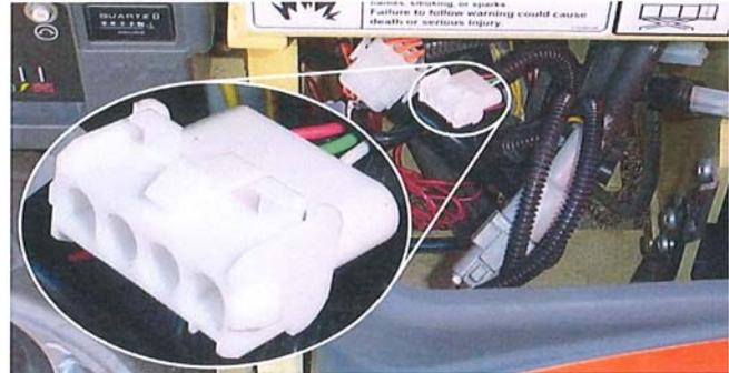
**Figure 3: Analyzer Connector**
