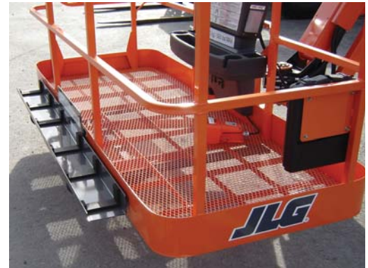
Due to the shift in the center of gravity caused by the tray installation the capacity combinations are required for factory approval. Removing the tray restores original machine capacity specifications.
