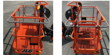
* Rail Extensions highlighted gray for images, actually orange in color
