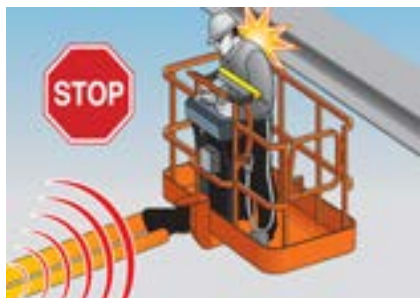
Horn sounds upon operator contact with the bar.
