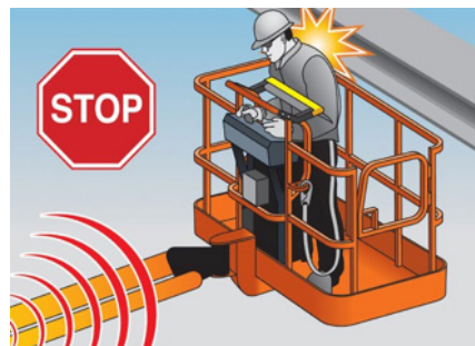
Horn sounds upon operator contact with the bar.
