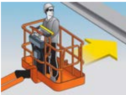
Operator moves toward obstruction.
