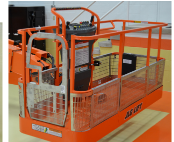
MESH TO MID RAIL
