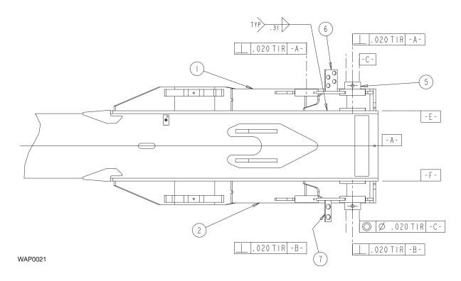
ORIENT, FRACTURE IN BEARING OUTER RACE, AT CLOCK POSITION SHOWN FOR EACH APPLICATION
