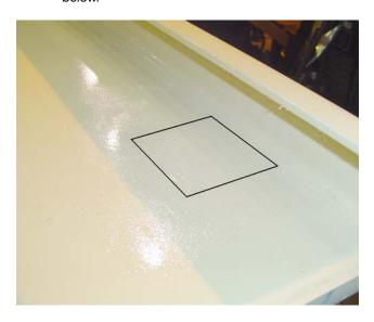
Using the plasma cutter, remove the square section of arm retainer channel' above kingpin as shown below. Do not discard removed section.
