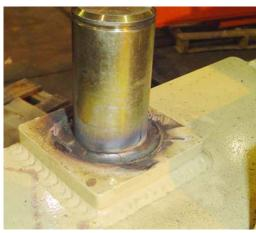
**NOTE:** Damage to the structural integrity of the metal may occur when heated in excess of 450°F (232°C). Use a surface thermometer to monitor the temperature of the discrepancy area.
