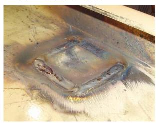
Arm retainer channel MUST be ground flush where removed section was welded to allow proper wear pad operation.
