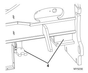
Use air carbon-arc equipment or a portable power grinder to remove the damaged rear axle mount weldments (4) from the frame weldment.
