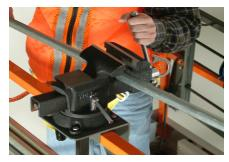
Used for clamping pipes to thread and cut, or hold other work materials. The vise is located at a height for comfort and ease.
