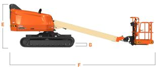
Platform Width 36-in / 91-cm A. Platform Length 96-in / 2.44-m В. Machine Width 7-ft 4-in / 2.23-m C. D. Tailswing 3-ft 2-in / 96-cm E. Machine Height 7-ft 7.5-in / 2.32-m E. Machine Length 24-ft 10-in / 7.57-m **Ground Clearance** 16-in / 41-cm
