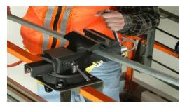
**Bench Vise** Used for clamping pipes to thread and cut, or hold other work materials. The vise is located at a height for comfort and ease.
