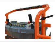
Old Style Platform No squares welded into the bar
