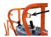
New Style Platform Squares welded into the bar
